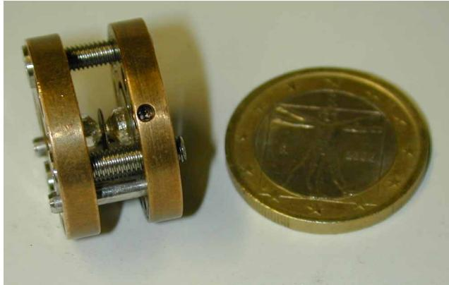
Figure 3. Lateral view of the Cu-Be DAC cell. Inside the cell the diamond anvil sets on the moissanite disks and the CuBe gasket are evident. The coin on the right is used for comparison.
