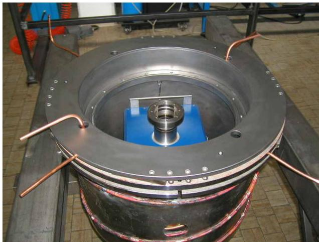
Figure 1. Photograph of the interior of the cryostat. Both the LN2 shield and the 8 T magnet are visible.
