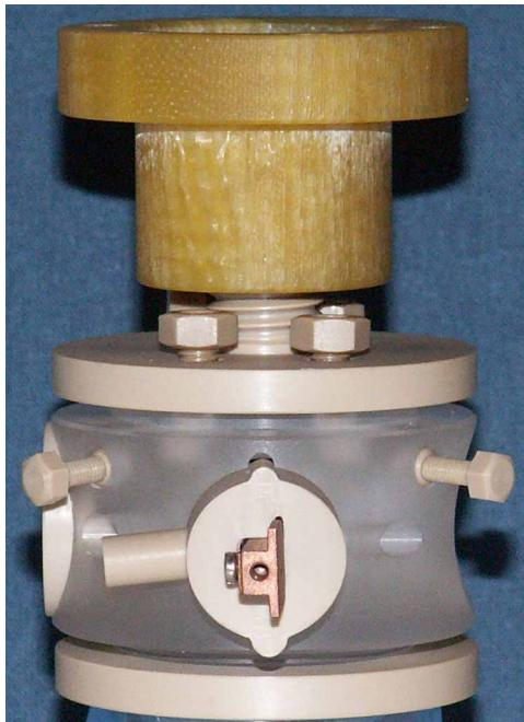
Figure 2. Photograph of the sapphire sample holder with its components in PEEK.
