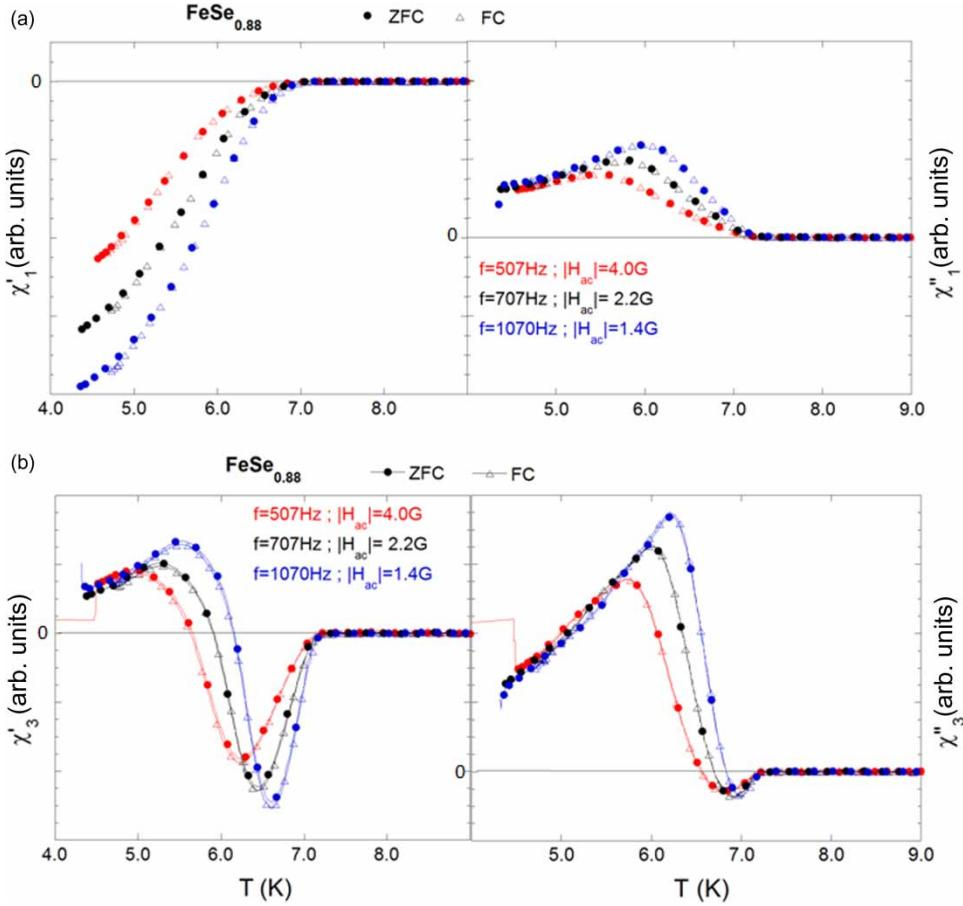
Figure 5. AC multi-harmonic magnetic susceptibility measurements of the  $\text{FeSe}_{0.88}$ : (a) real and imaginary parts of the first harmonic; (b) real and imaginary parts of the third harmonic. For comparison, all graphs are plotted to the same scale.
