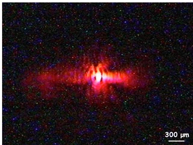
Figure 4. Image of the focal spot produced by the Cassegrain optical system, with a horizontal collimated illumination. A similar image is obtained for the vertical focus. The observed spot has a diameter  $<300\ \mu\text{m}$ .
